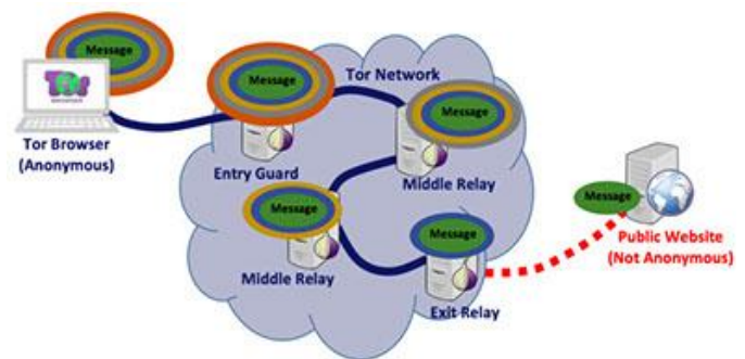
Image 3. A representation of an onion routing network or tor network as a cloud of nodes from the outside (source: https://www.axontechnologies.com/images/1_0zdvagxjbzdom2nrtr0zq393x196.jpg?crc=376330005 )
